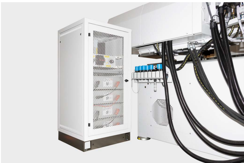
Fig. 4: Super-caps to cover brief load peaks
