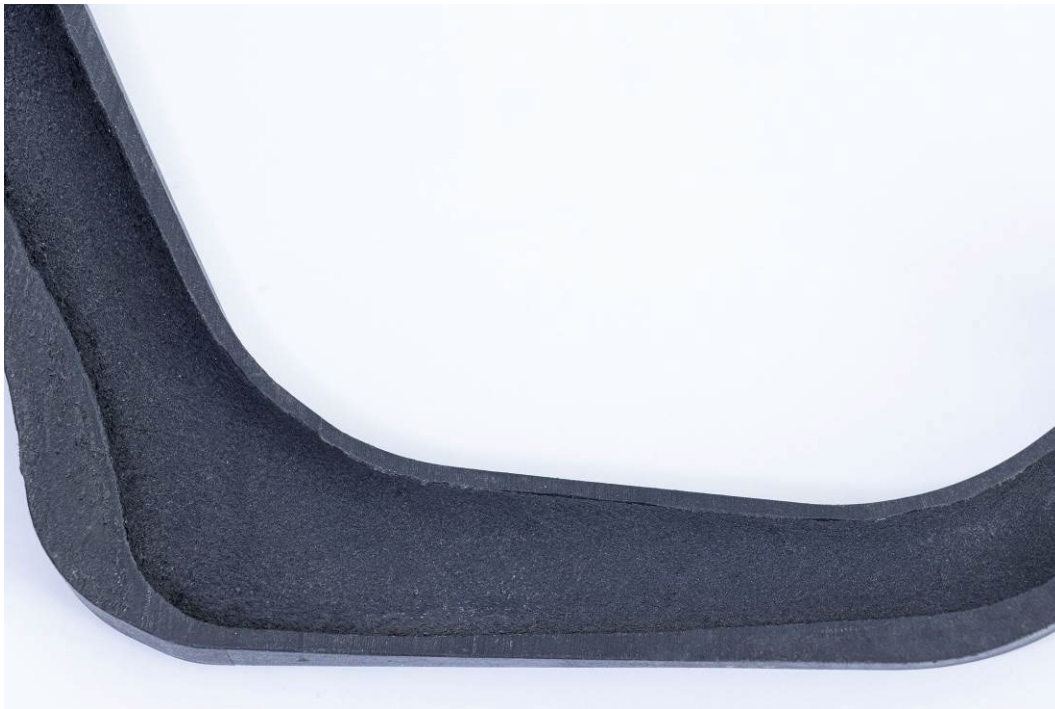
Fig. 4: Airmould channel on gas pedal
