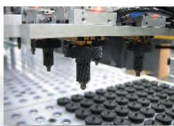
WITTMANN sprue pickers and servo robots are ubiquitous in plastics processing; typically used for part insert operations, part removal and are generally essential in any part of the injection molding process.
