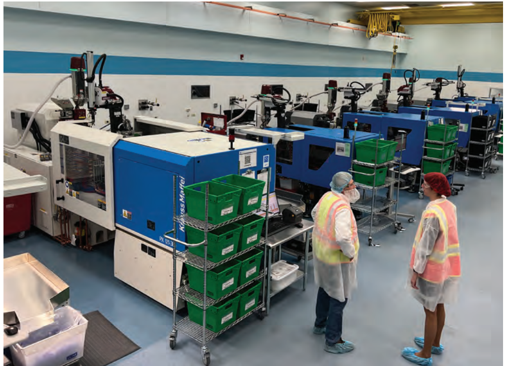
Westfall Technik's Antioch, IL plant uses WITTMANN robots and sprue pickers for consistent, reliable parts removal.
