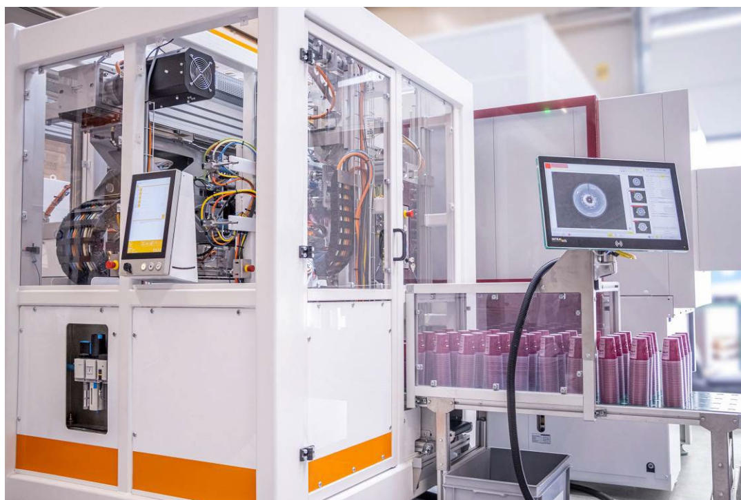
Fig. 3: IML line of BECK with INTRAVIS vision system
