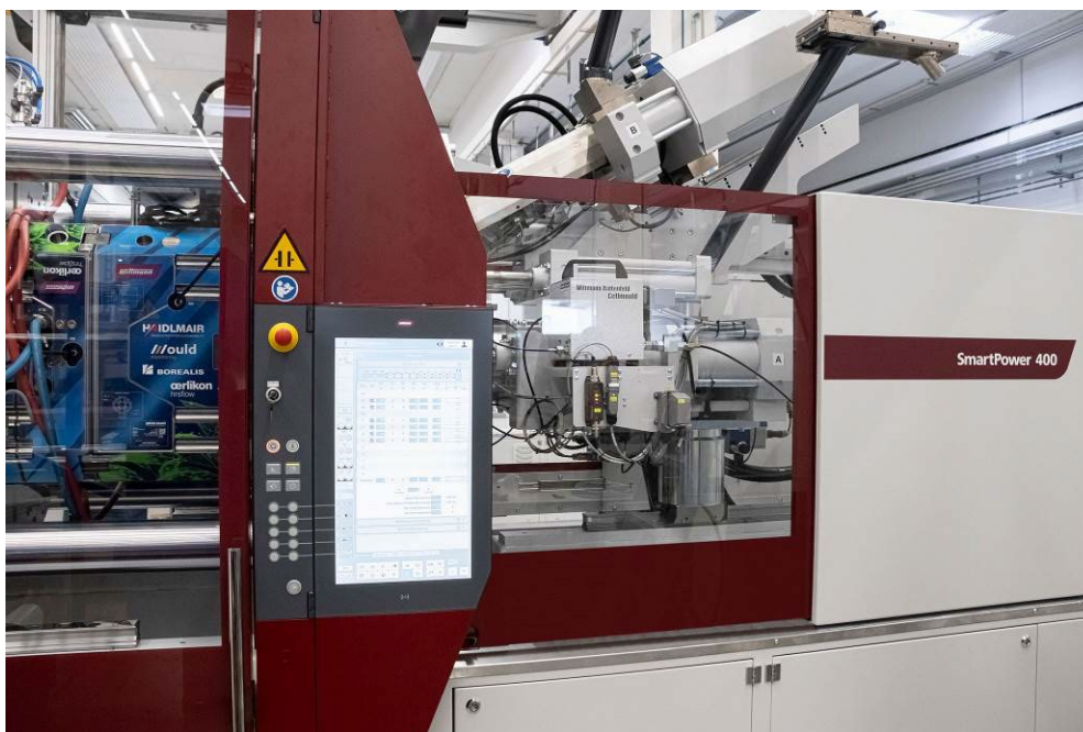
Fig. 2: 3 component machine equipped with Cellmould technology
