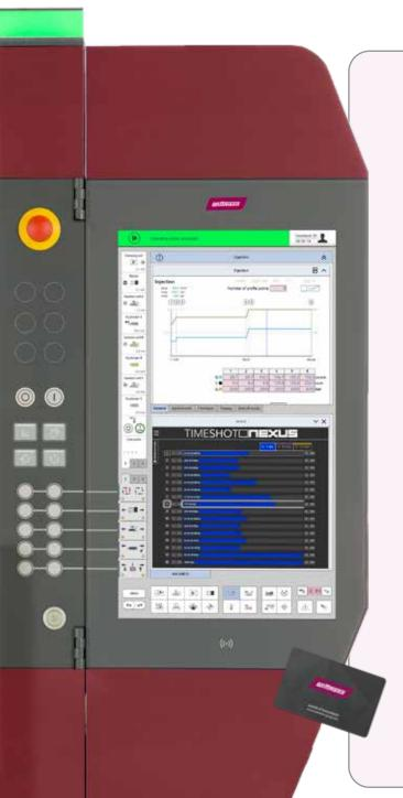
For parameter setting and regulation, monitoring and documentation of the LIM injection molding process, an optional program module is available to complement the standard machine control system.
