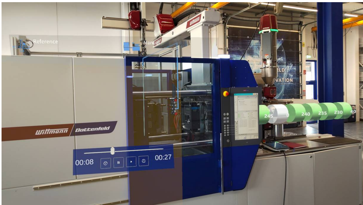
Fig. 1: Augmented barrel temperatures starting from nozzle temperature down to feed temperature (from left to right); fade-in and animation of the robot's future program.
