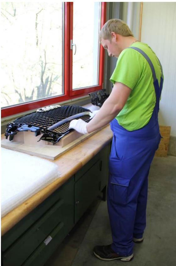
Fig. 5a + b: Assembly work on an Audi radiator grille and finished parts
