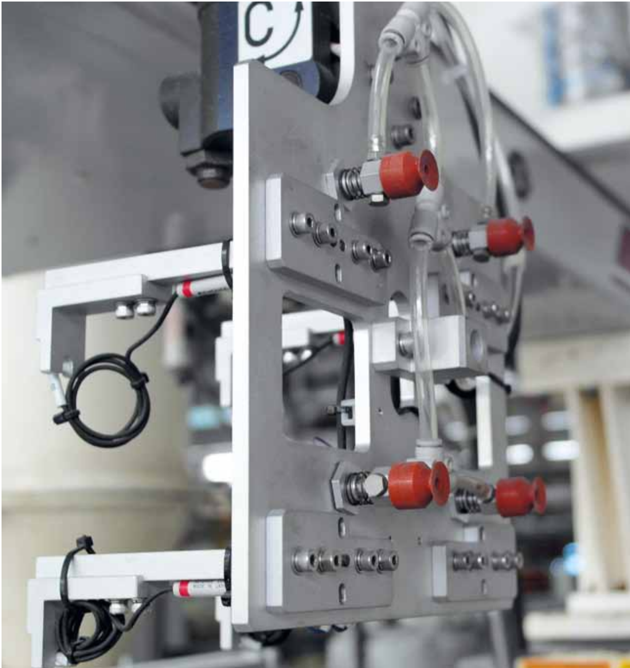
Greenland customized end-of-arm tooling (EOAT), designed by WITTMANN BATTENFELD Singapore.
