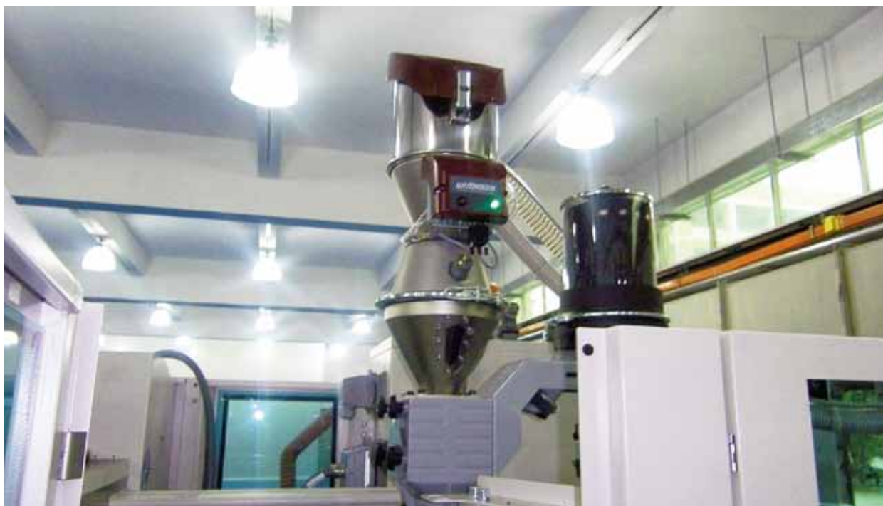
WITTMANN FEED-MAX material loader, mounted on an injection molding machine.
