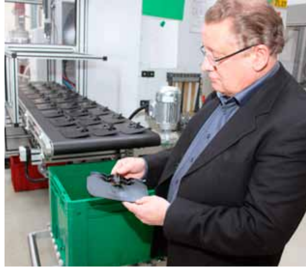
Dieter Diekmann checks anti-surge baffles. Picture left: This anti-surge baffle with flow-relevant naps is made of flexible material to facilitate insertion into the fuel tank. Picture right: In virtual "ghost shifts", hundreds of thousands of these automotive parts are produced from modified HDPE.
