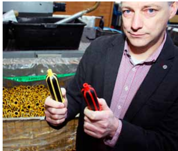
Picture left: Liesa Feikes, third-year trainee mold maker, selects a graphite electrode. The processor based in Leer manufactures these eroding components itself. Picture right: Two-component technology in different colors for electrical appliances: Holger Meyer, Deputy Plant Manager, presenting two handles for flashlights made of LDPE and colored TPE.
